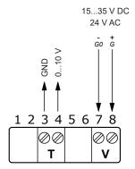
GND and G0 are internally connected.
