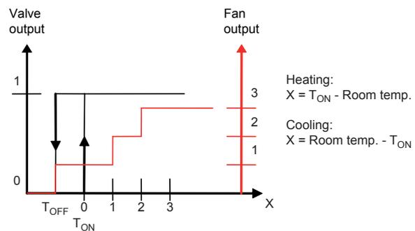
When there is no heating or cooling demand in the Auto position, the fan will run at its lowest setting. This can be changed to make the fan stop when there is no heating or cooling demand. The fan is also deactivated when in modes Off and Window. However, it will continue to run if mould protection has been configured.
