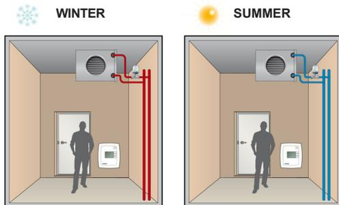
In 4-pipe installations, there are two separate water systems for heating and cooling with separate valves. The thermostat uses two outputs for control of heating and cooling in sequence.
