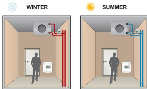
In 4-pipe installations, there are two separate water systems for heating and cooling with separate valves. The controller uses two outputs for control of heating and cooling in sequence.
