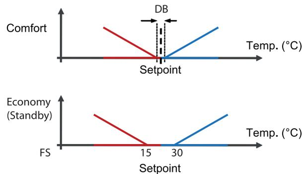
The above figure of the control principle show the corresponding requirement of the controller function. This requirement is recalculated by the controller to a value for the actuator output, depending on the selected output function.
