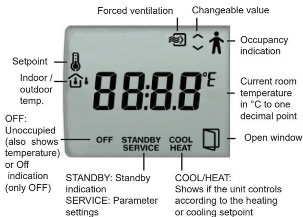
The buttons on the controller enables easy setting of parameter values using a parameter menu shown in the display. The parameter values are changed with the INCREASE and DECREASE buttons and changes confirmed with the Occupancy button.
