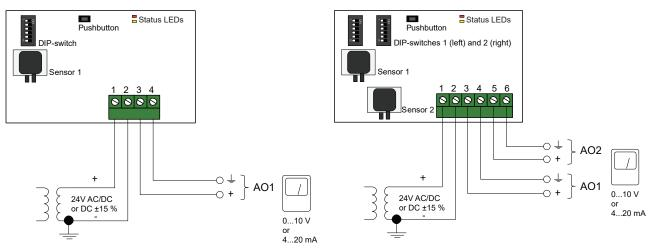
Fig. 1: Wiring for models with one sensor
