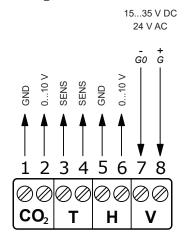
GND and G0 are internally connected. The PT1000 sensor can either be connected via a separate signal neutral or to GND or G0 using a jumper.
